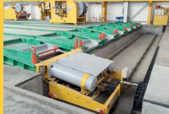
Stressing and detensioning of the steel wires
