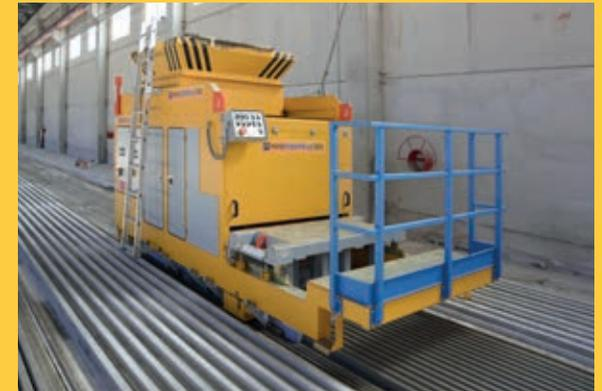
Element casting, Wet Casting WF
